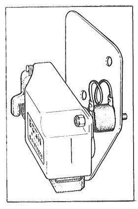
O NOTE: When mounting the electronic box (p/n 420 264 470 aluminum body) be sure to use the previously mentioned ground wire.
