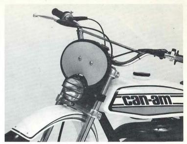
The Enduro lighting system uses a tough, rubber-mounted head and taillight and a rugged solid-state electronic voltage regulator.
