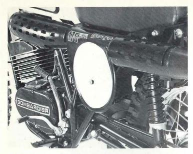
The new Can-Am 175 T'NT O/R has the basic features which have made Can-Am highly competitive on track and trail, including ultra-slim Bombardier-Rotax rotary-valve engine and variable volume multilube injection system.
